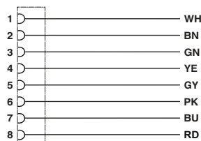
S/A cable: M 12 connector/socket on free conductor end
