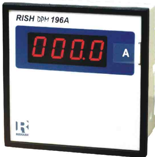
RISH DPM 196A 1PH. current measurement (AC)
